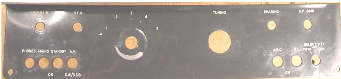
Above: fingerplate off an S.940 before any restoration work – note the heavy scoring associated with the bandswitch and typical circular scratches around the other control cut-outs (especially the RF gain)
